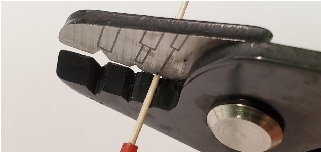
Figure 7. Cut through the LCP with the 250um to 125um Hole.
