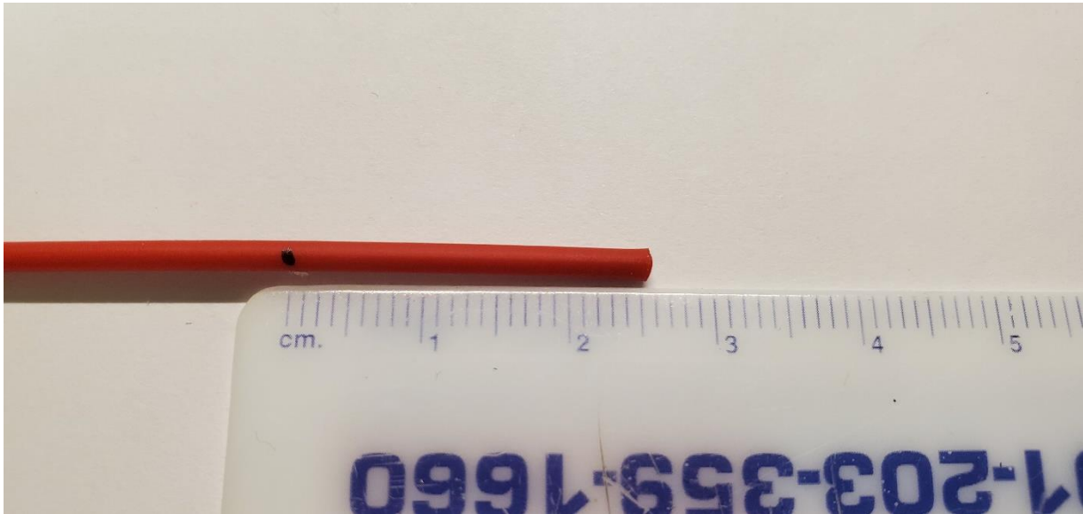
Figure 3. Cable Outer Jacket Marked 25 mm from End
