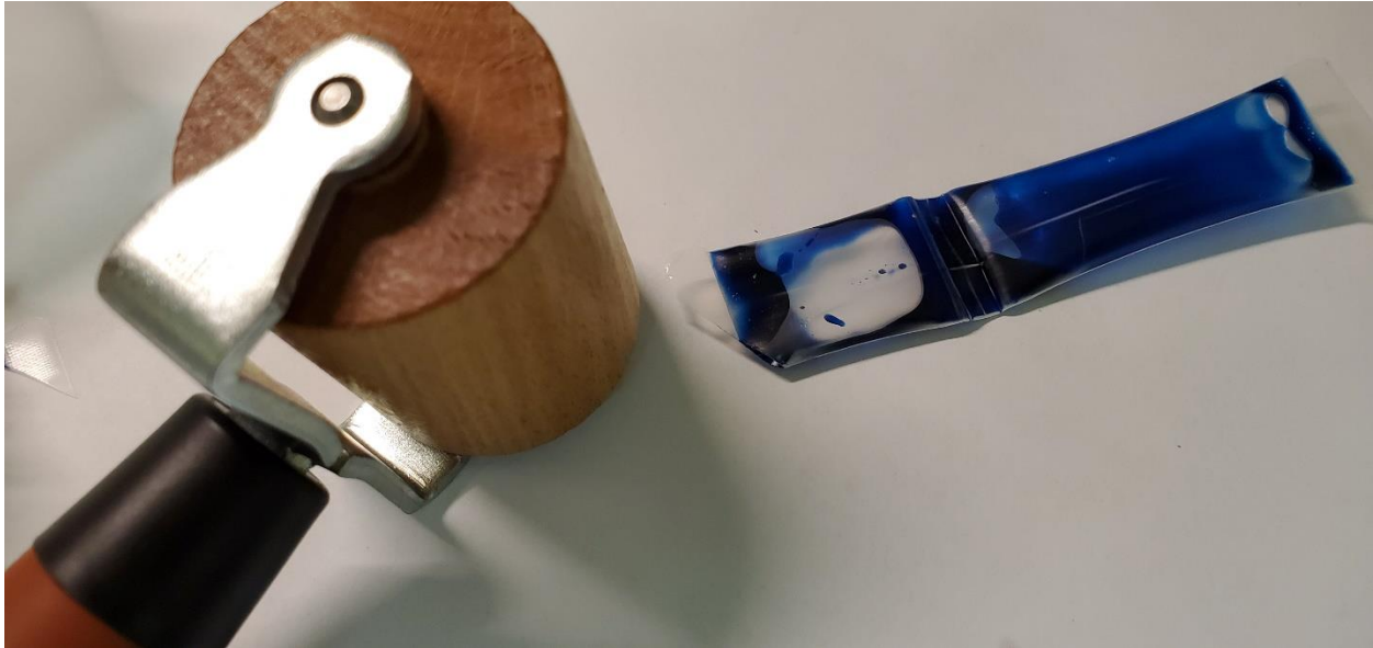
Figure 9. Epoxy Bi-Pak Mixed with Roller
