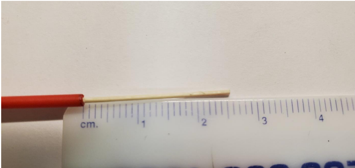
Figure 5. 25 mm of Outer Jacket Stripped
