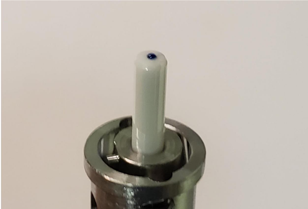
Figure 11. Epoxy Bead at the Tip of the Connector Ferrule
