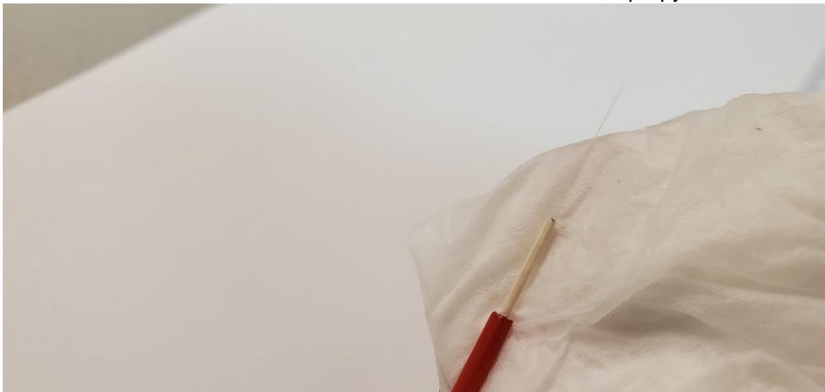
Figure 8. Remove all Traces of Buffer from Fiber Using Lint-free clothe and IPA
