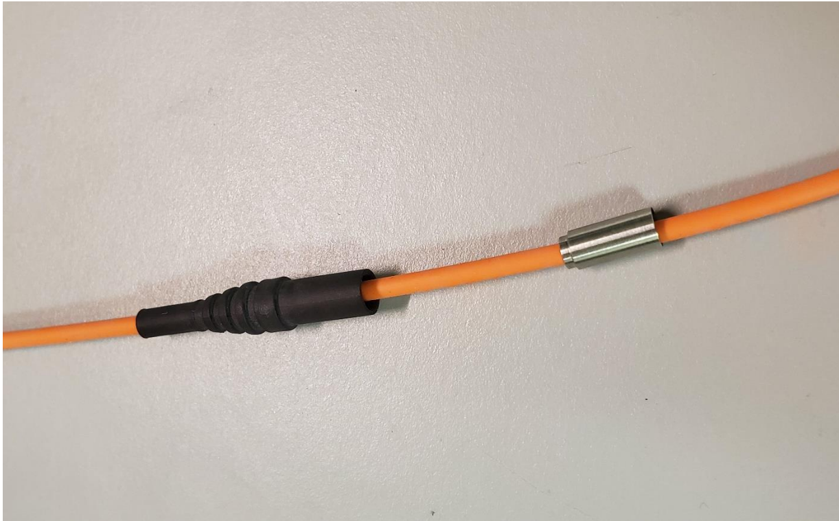
Figure 2. Boot and Crimp Ring on Cable prior to Termination
