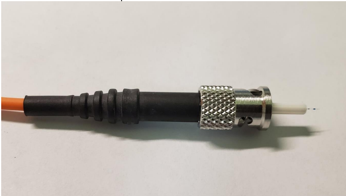
Figure 15. Boot in Place
