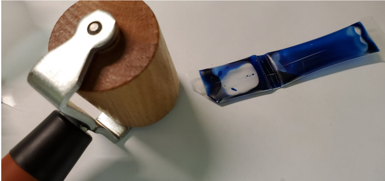
Figure 8. Epoxy Bi-Pak Mixed with Roller
