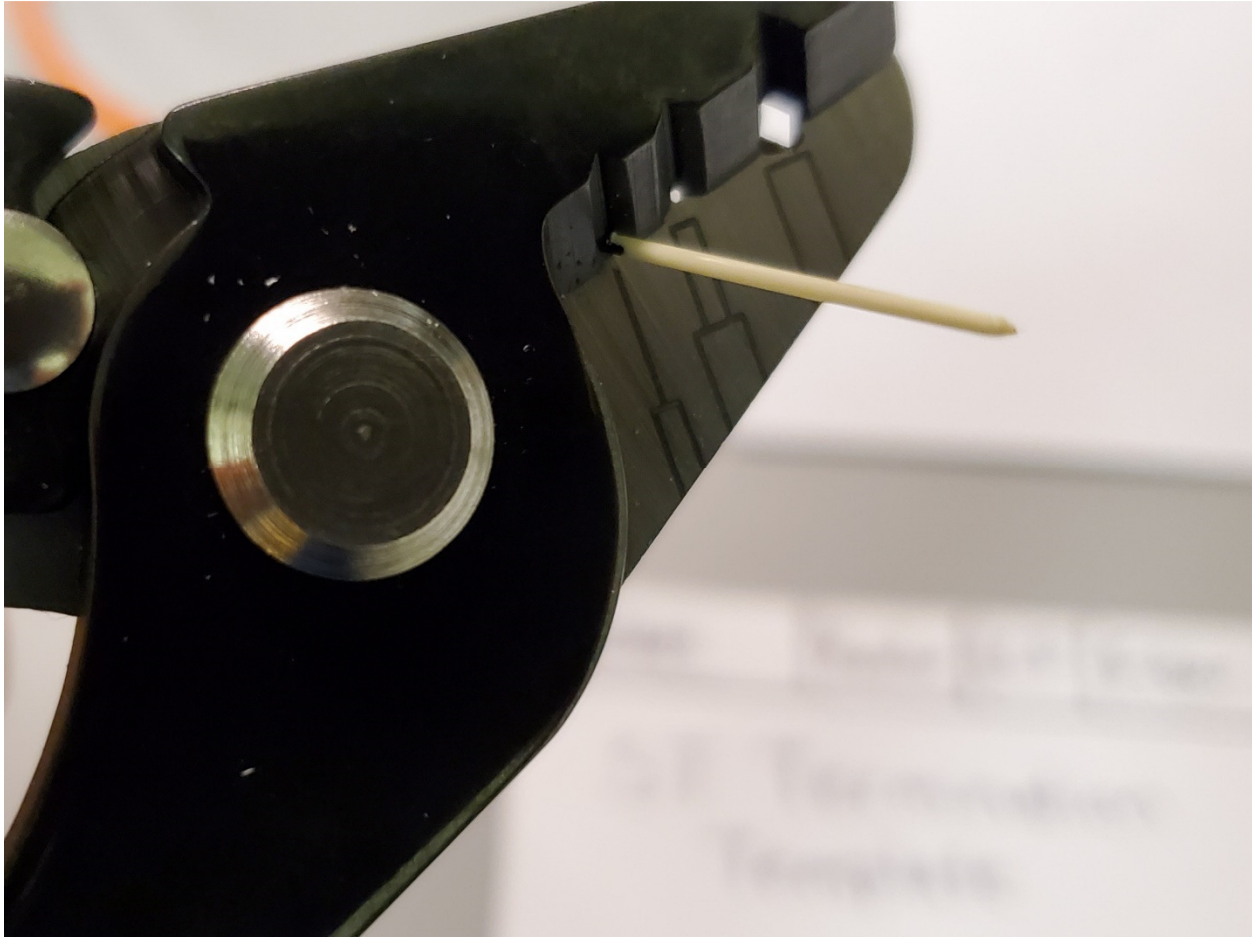
Figure 7. Stripping the LCP Layer
