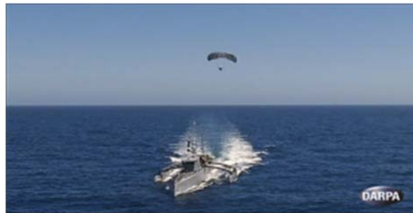
Figure 4. TALONS Kite with Linden Photonics Hybrid Tether
