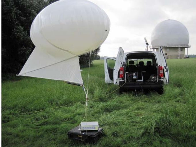
Figure 7. Kite Aerostat Using Tether with 2 Kevlar Strength Members in Parallel.
